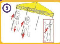
Lift each leg until the Ring Pull snaps into the first hole
