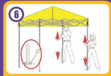
For height adjustment, place your foot on each leg footpad and slowly extend each leg to desired height.
