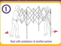
Grasp the lower "V" at centre Truss Bar. Lift and pull the frame half way out.
