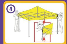
Now that Frame is fully expanded. Push Sliding leg Brackets upwards until Ring Pull Pin locks into position on each leg.
